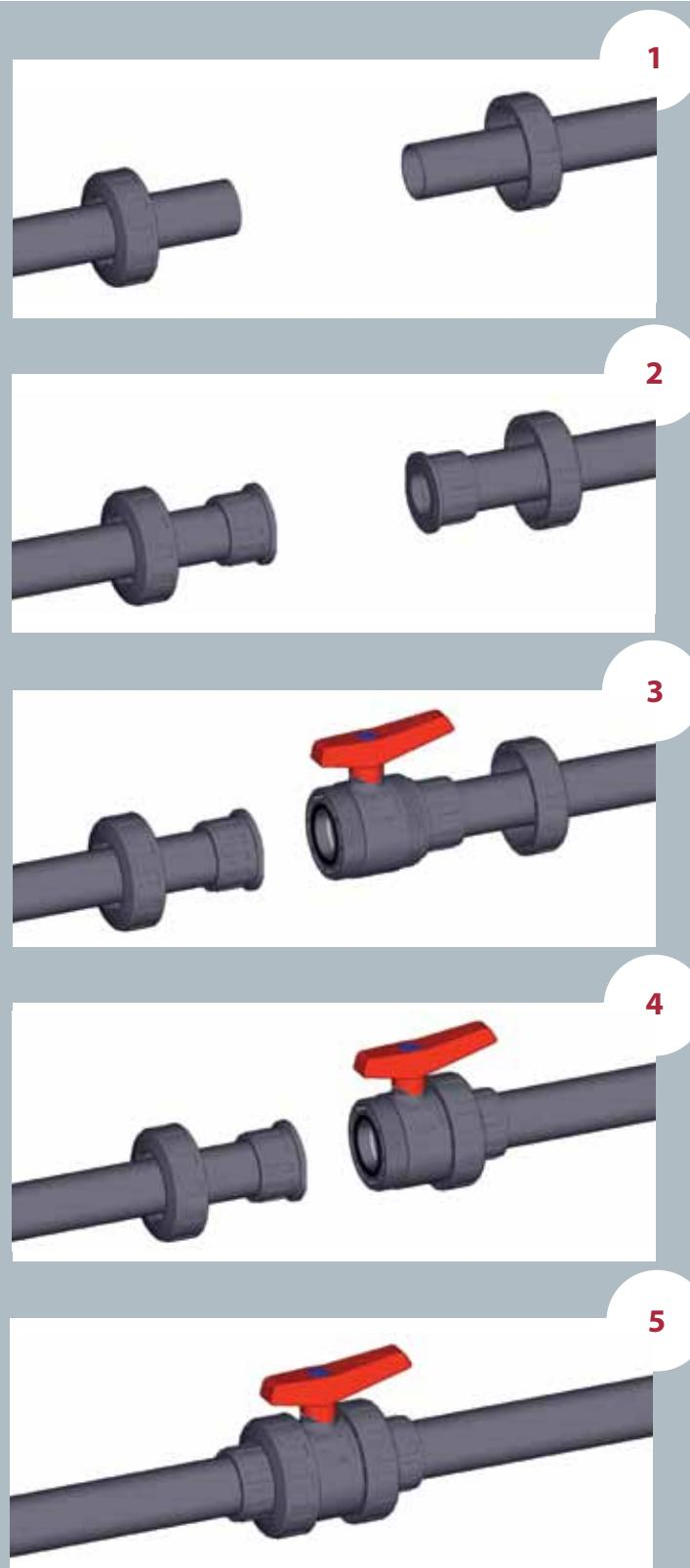
**SEAL-CARRIER****Industrial Series - Threaded seal-carrier**
