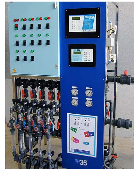
Automatic fertirrigation system
