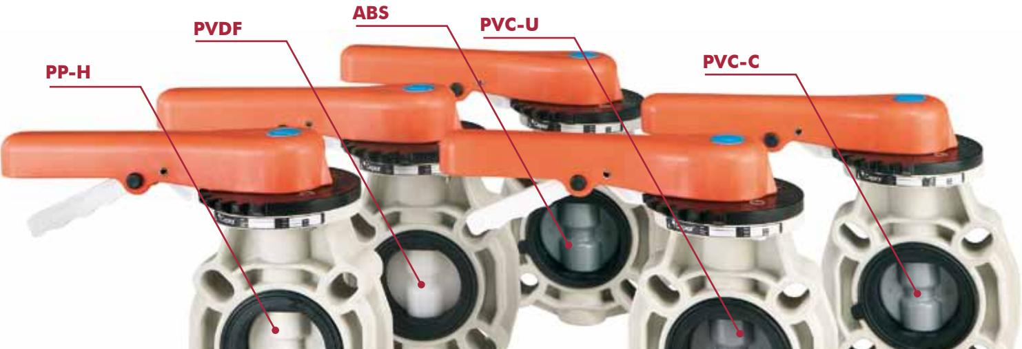
New range of butterfly valves in its Industrial Series (stainless steel shaft, food grade EPDM or FPM sealing, PP - GF body & disc available in several materials). Sizes from D63 up to D315 (2" to 12"). The valve represents a major step forward both for its design and new features, offering the following characteristics:
